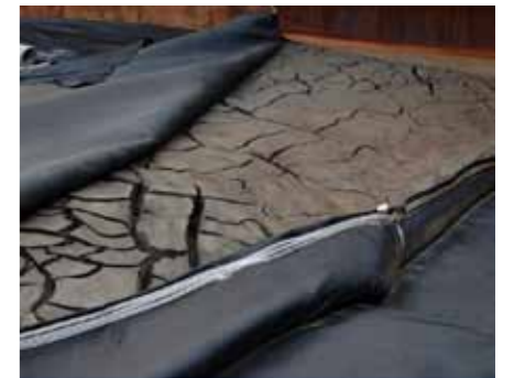
Dewatered contaminated sediment inside holding barge
