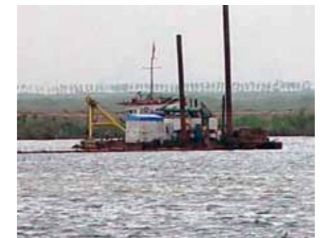
Medium scale hydraulic dredge
