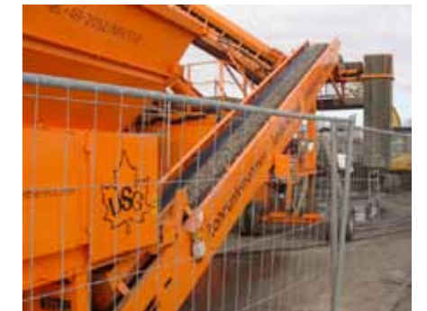
Separation of aggregates from contaminated slurry fines
