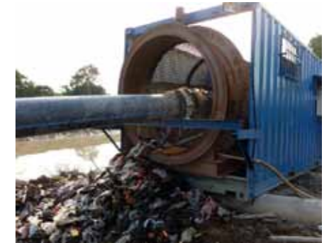
Separation of trash from contaminated sediment slurry
