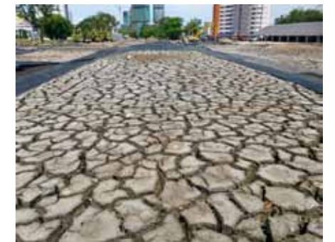
State of contaminated sediments following Geotube ® dewatering
