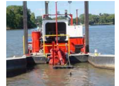
Small scale cutter-suction dredge used to accurately dredge contaminated sediment layer
