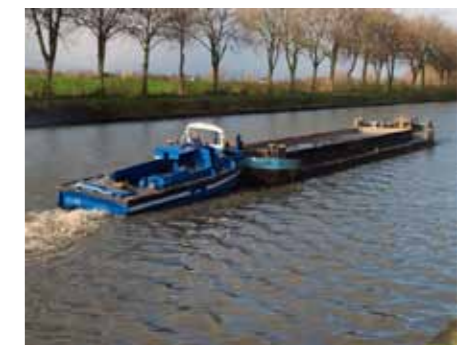
Transport of contaminated sediment to dewatering site
