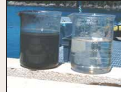
Aquaculture benthic deposit water before and after Geotube® treatment.
